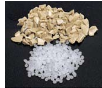
High density polyethylene starts as polymer resin (foreground). It is formed under high pressure to create dense, solid plastic sheets for manufacturing into locker components. Waste material from the process is immediately recycled (background) to make new sheets.
